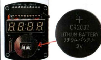
8、装上纽扣电池。(平面+极朝上) Install the button cell battery. (Planar + Extreme Upward)
