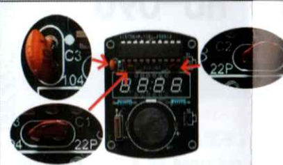
4、焊接 22PF 和 104 瓷片电容。 Solder 22PF and 104 ceramic capacitors.
