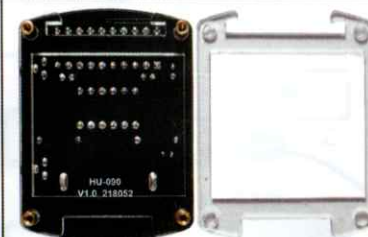
12、将对应图片外壳装在电路板背面。 Mount the corresponding picture shell on the back of the circuit board.
