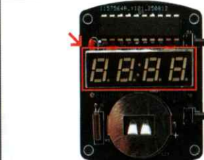
7、焊接数码管。(注意数码管方向) Solder digital display tube. (Pay attention to the direction)
