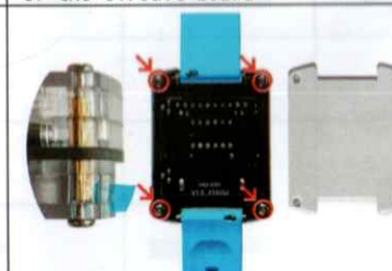
15、将对应图片外壳装上，并用 M2 螺 丝进行固定。 Install the corresponding picture shell and secure it with M2 screws.
