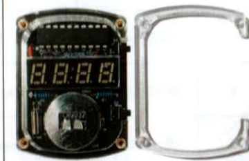
10、将对应图片的两片外壳装在电路板 正面。 Install the two corresponding shell pieces of the picture onto the front of the circuit board
