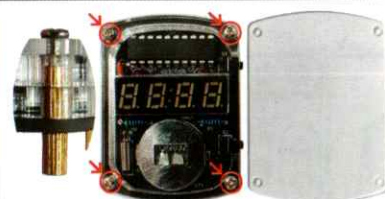
11、将对应图片外壳装上，并用 M2 螺丝 进行固定。 Install the corresponding picture shell and secure it with M2 screws.
