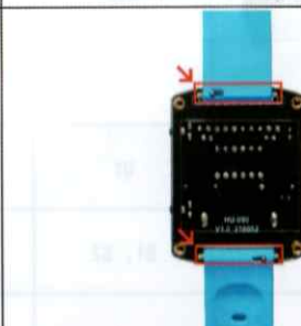
14、将表带装到外壳的凹槽中。 Install the watchband into the groove of the case.
