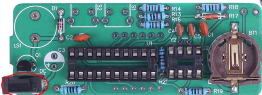
Step 14: Install 1pcs 32.768K Crystal Oscillator at Y2.
