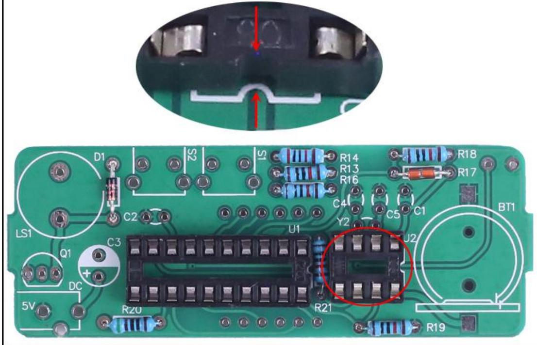
Step 9: Install 2pcs 5pF Ceramic Capacitor at C4,C5.
