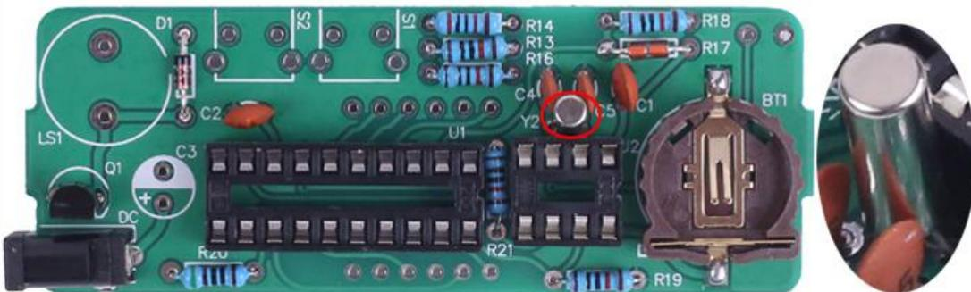
Step 15: Install 1pcs 100uF Electrolytic Capacitor at C3. Pay attention to distinguish between positive and negative. The shorter pin is negative pole and insert into white pad.
