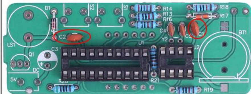
Step 11: Install 1pcs CR1220 Battery Socket at BT1.
