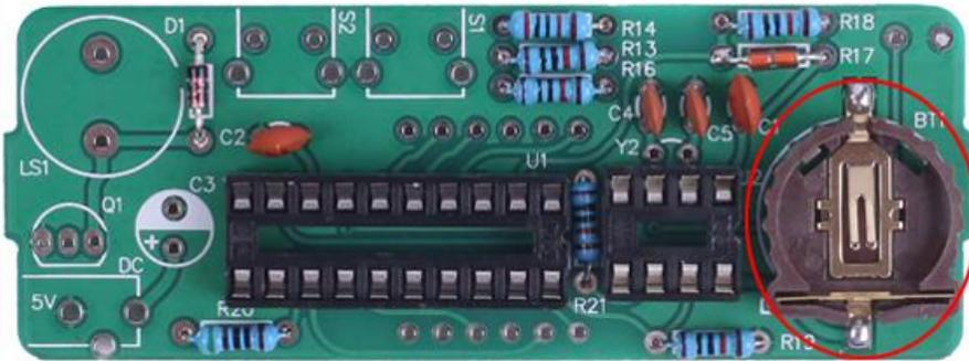
Step 12: Install 1pcs TO-92 S8550 Transistor at Q1. Pay attention to the installation direction of arc.
