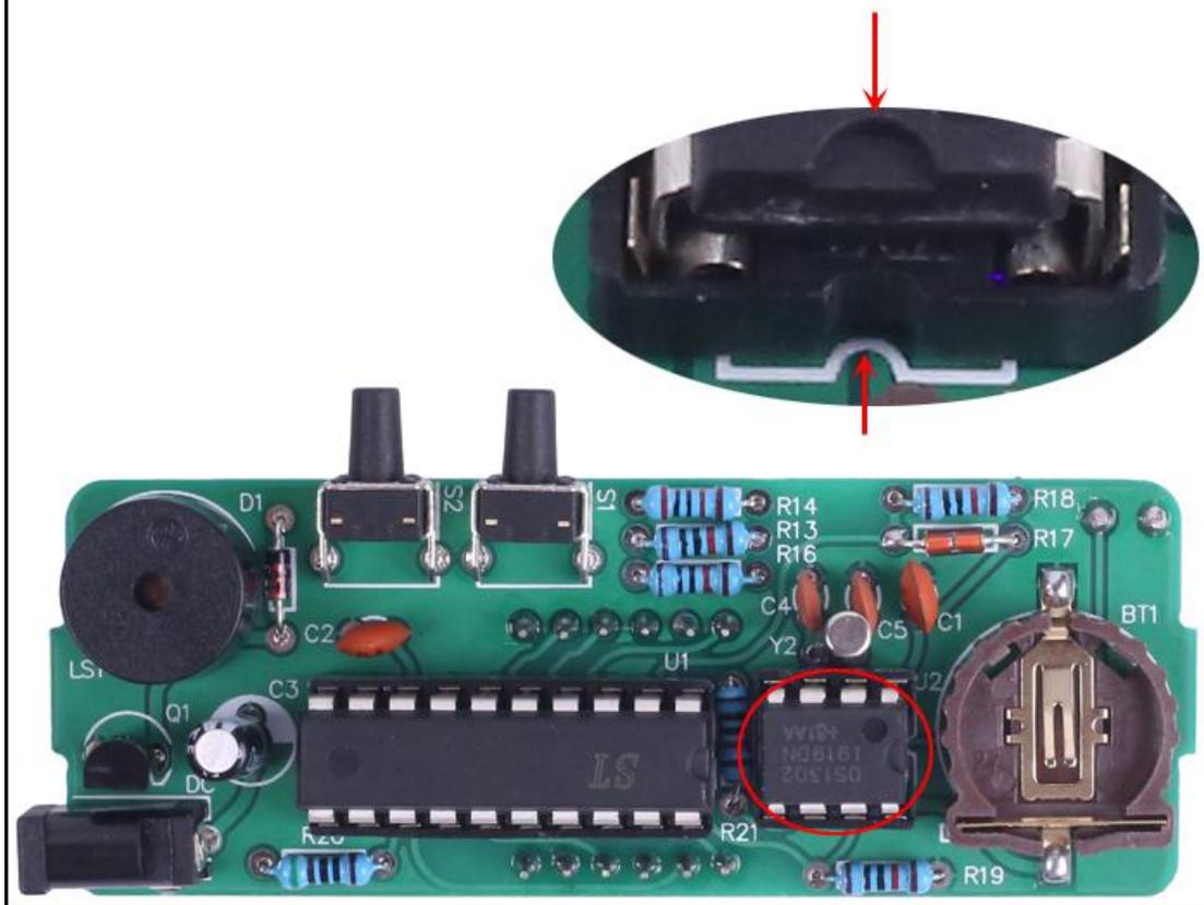
Step 21: Install 1pcs 3V CR1220 Battery on battery socket. Pay attention to the direction of the battery.
