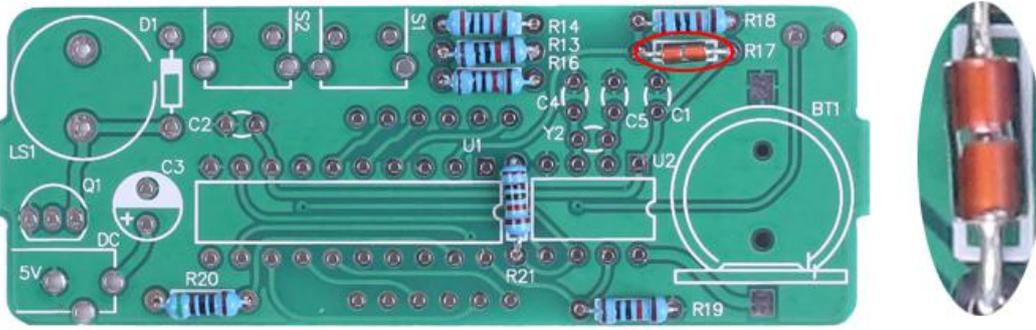
Step 5: Install 1pcs DO-35 1N4148 Diode at D1. Pay attention to the installation direction. Note: The black mark on Diode and the white mark on PCB are corresponding.
