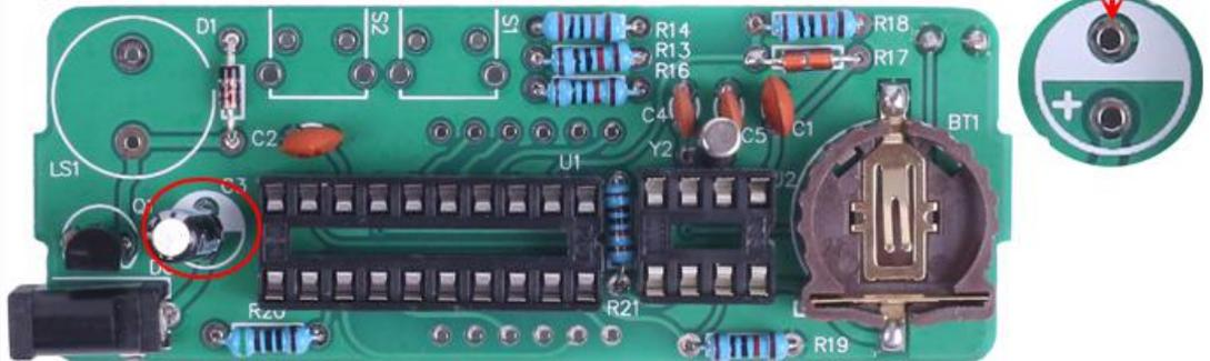
Step 16: Install 1pcs Passive buzzer at LS1. Pay attention to the installation direction.
