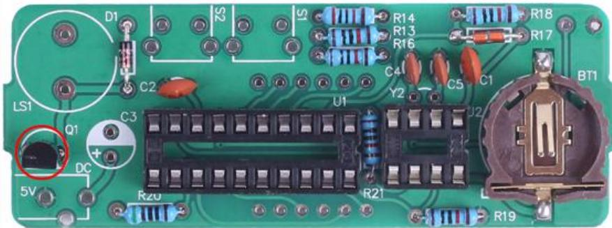
Step 13: Install 1pcs 3.5\*1.2mm DC Power Socket at DC.
