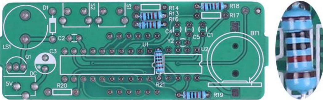
Step 2: Install 1pcs 20Kohm Metal Film Resistor at R14.
