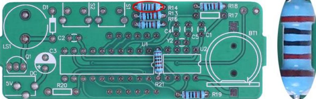
Step 3: Install 1pcs 510ohmMetal Film Resistor at R20.
