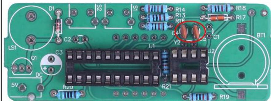
Step 10: Install 2pcs 0.1uF 104 Ceramic Capacitor at C1,C2.
